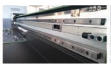
THK silent dual rail high-speed printing effectively reduces the mechanical noise generated in the output process and improves the high-quality working environment
