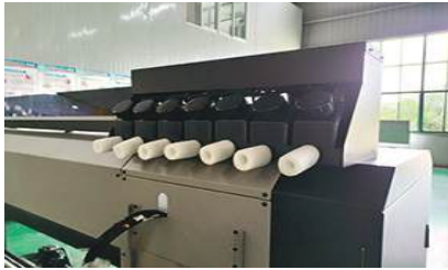
1.5L bulky ink bottle with lack of ink alarm system represents advanced concept of the industrial application
