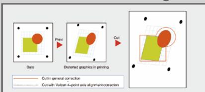
The Vulcan FC-500VC efficiently handles materials loaded on a slant and also compensates for size/shape distortions. Precise and accurate cuts are assured with our proprietary four mark high-tech detection algorithm.
